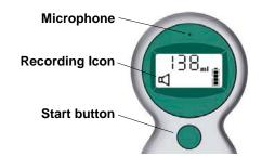
2. The microphone is located just above the display. Hold the microphone approximately 6 inches (15 cm) from your mouth when you are recording the annotation, and speak clearly.
