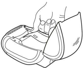
7. The Label Writer feeds the labels, stopping at the beginning of the first label. If the Label Writer stops without feeding the label, make sure the label is fully inserted and then press the form-feed button. Close the top cover.
